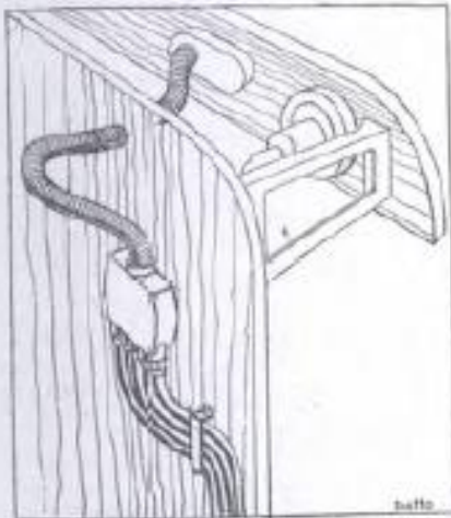
The neat installation of the electrical connections on the 25 h.p. Diatto chassis
